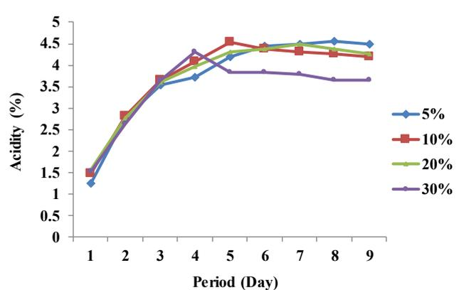
**Figure 07:** Formation of acetic acid during fermentation with different inoculums size
